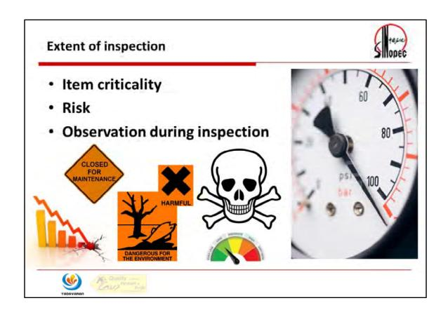
The extent of inspection is related to the item criticality and Risk. The criticality rating of the equipment for each package is mentioned in a document with the same name "criticality rating". Also, service fluid, working pressure/temperature, location, etc. shall be considered.
